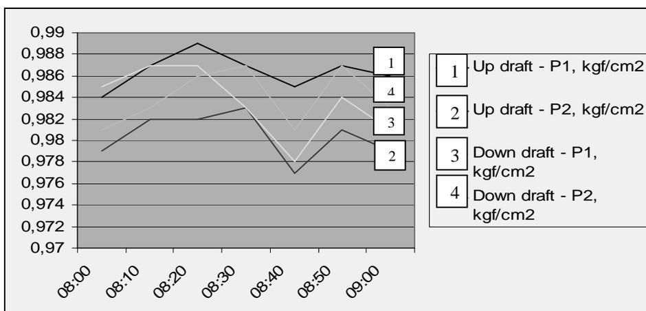
Fig.7. Inlet air pressures - for up and downdraft modes
