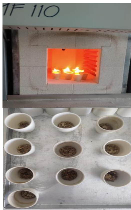
Fig. 6. Ignition Rate Testing temperature and duration, establishing a clear hierarchy of fuel quality.
