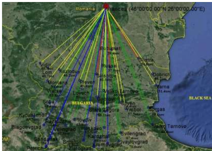
Fig. 4. The travel times t_s-t_p (Vrancea source) show the time for reaction after the early warning is issued
