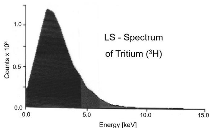
Fig.3. Liquid scintillation spectrum of the  $^3H \rightarrow ^3He$  decay, measured in the LS spectrometer.
