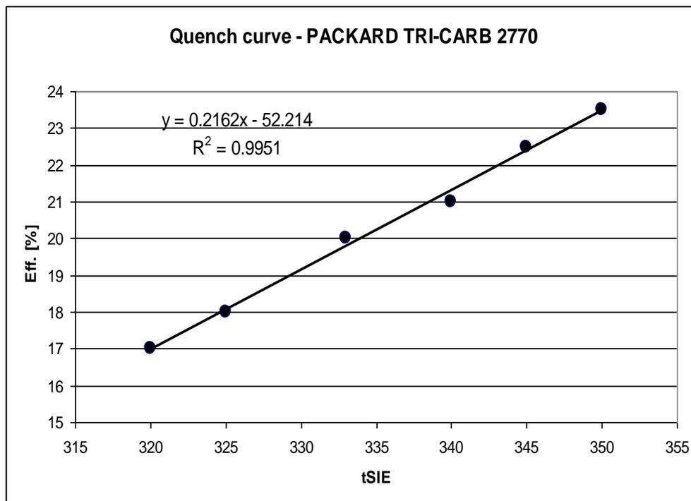
Fig. 4. Quench curve for  $^3\text{H}$  using tSIE as quench indicator
