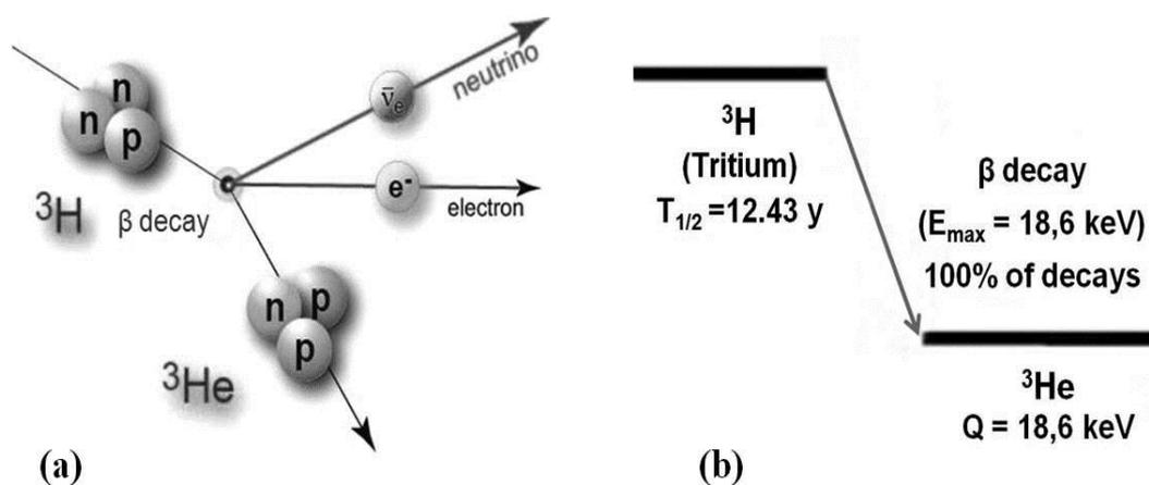
Fig.1. a) Disintegration of tritium ( $^3\text{H}$ ) in helium-3 ( $^3\text{He}$ ); b) in the process only electrons ( $E_{\text{max}} = 18.619 \text{ keV}$ ), emitted from the  $^3\text{H}$  nucleus can be detected. The total energy of the radioactive decay is statistically distributed between the electron and the neutrino, the latter one not detected in the LS spectrometer.
