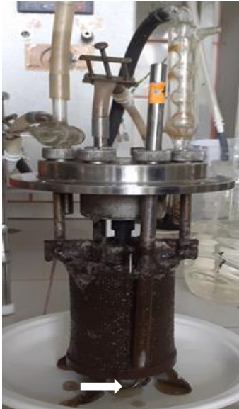
Fig. 9. The steel mesh carrier with immobilized microbial consortia (white arrow) after 30 days of operation.
