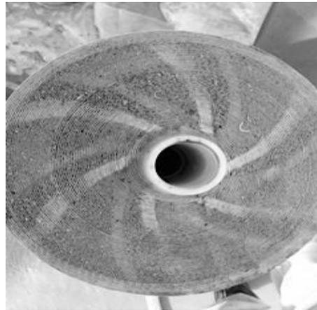
Fig. 4. Polyamide conventional membrane clogged with fouling
