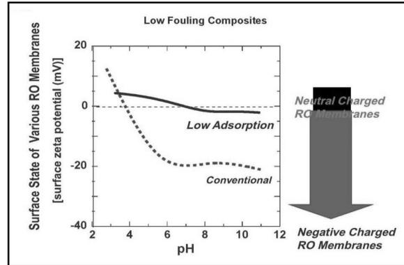
Fig. 5. Change of the potential of conventional and SLFM membrane surface at different pH
