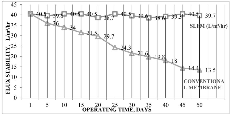
Fig. 3. Flux change through the filtration cycle
