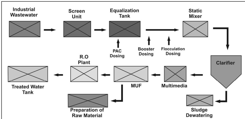
Fig. 1. Technological schema of wastewater treatment process in RAK, U.A.E
