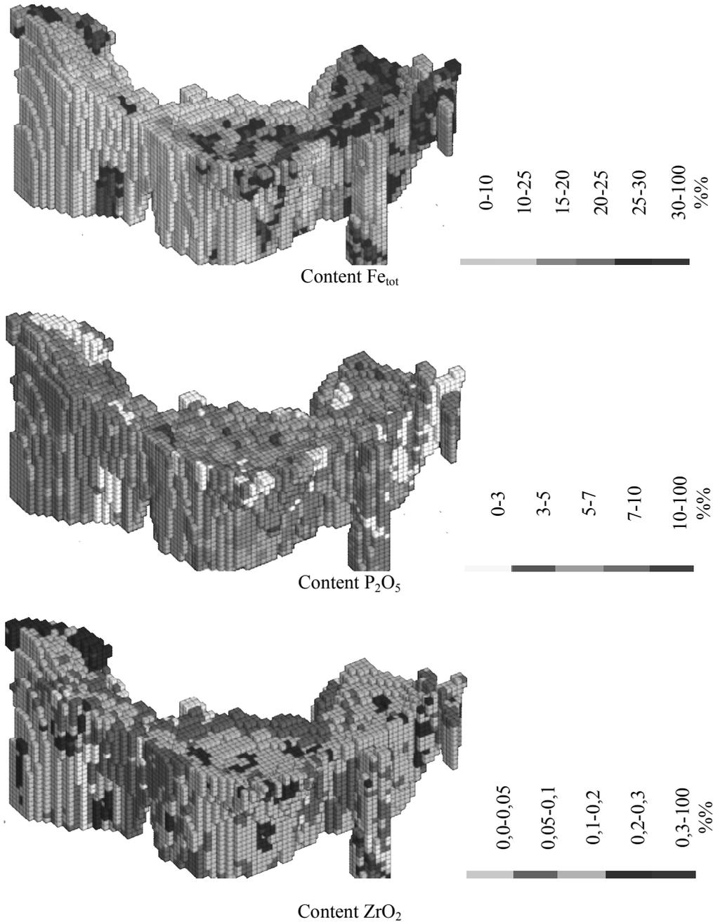
Fig.2. Differentiation by content and reserves of principal components of baddelite-apatite-magnetite deposit, perspective apatite-shtafelyte and apatite-carbonatite deposits of the Kovdor ore cluster made by 3D digital model
