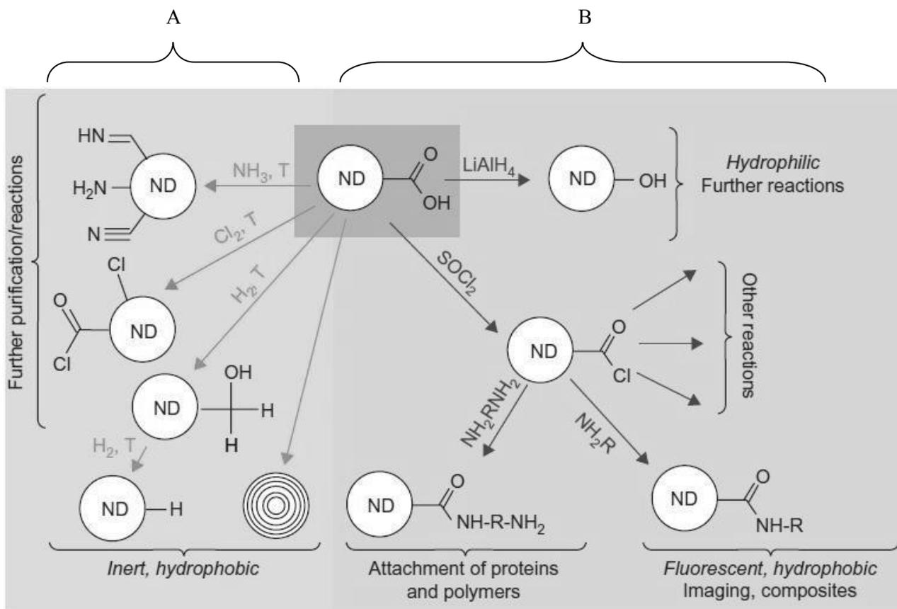
Fig.1. NDs with attached carboxylic groups (NDS-COOH). The surface of NDs-COOH can be modified by means of high-temperature gas processing (area A) or by means of temperature independent chemical reactions (area B) [14]
