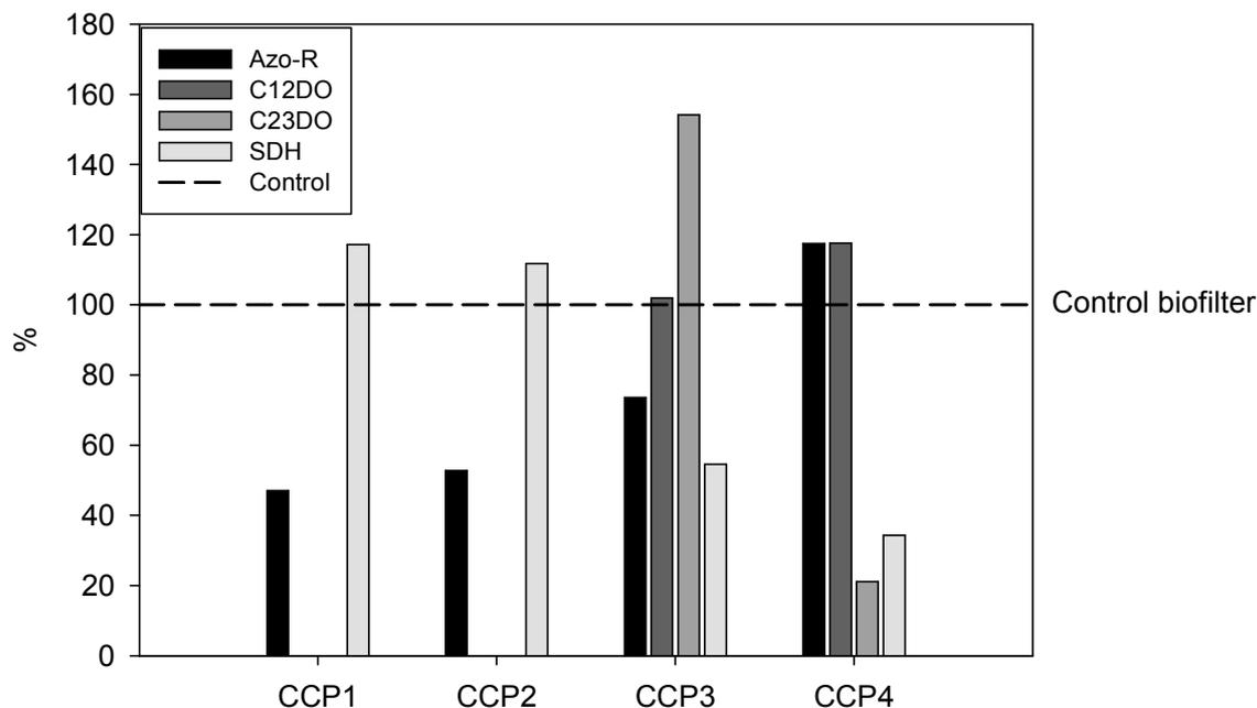
Fig.7. Effect of NDs on the enzymological indicators: Azo-R (azo-reductase); C12DO (catechol-1,2-dioxygenase); C23DO (catechol-2,3-dioxygenase); SDH (succinate-dehydrogenase) at four CCPs in biofilter with added NDs. The values for control biofilter are 100%.
