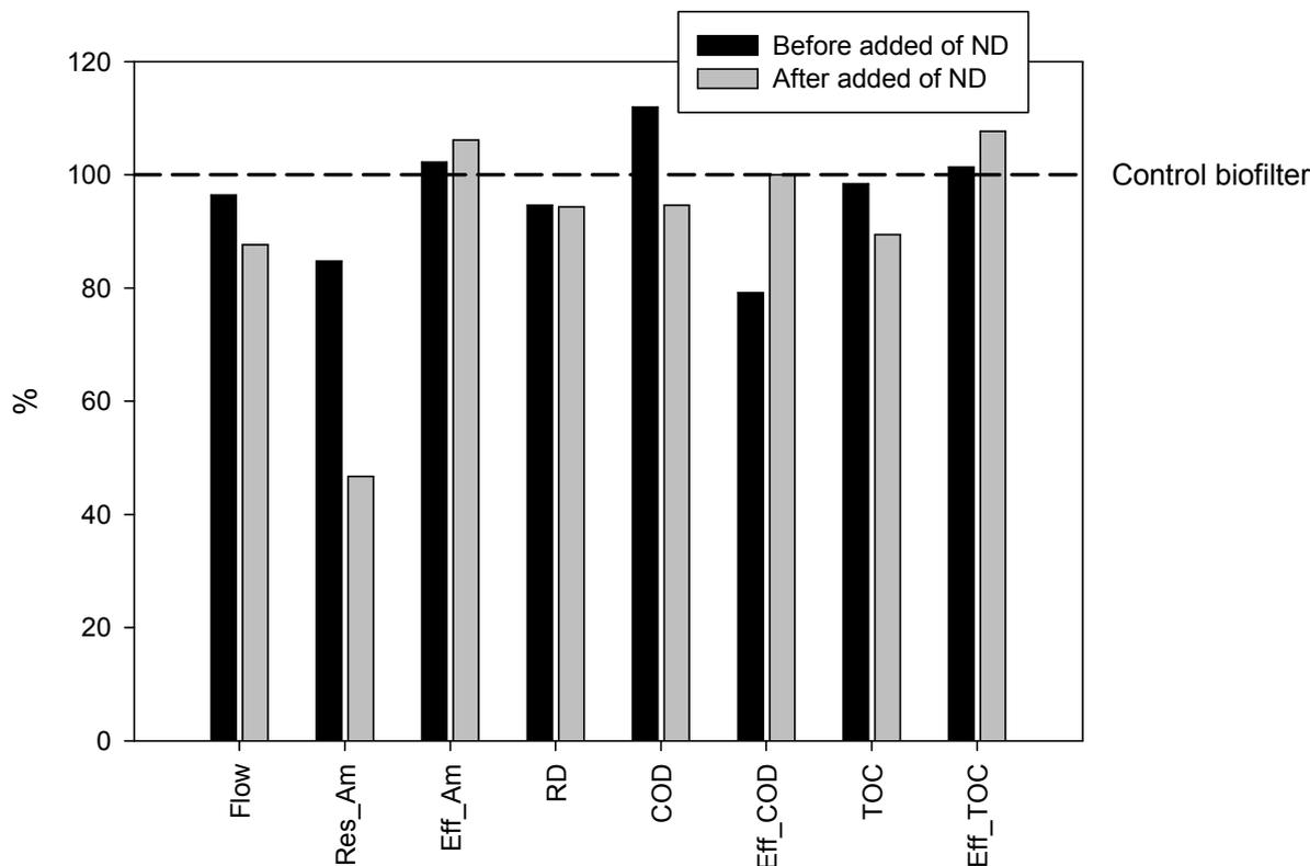
Fig.3. Effect of NDs on the technological parameters of the process in biofilter with added NDs: Flow, Residual amaranth (Res\_Am); Effectiveness of amaranth decolorization (Eff\_Am); Amaranth decolorization rate (RD); COD; effectiveness of COD decreasing (Eff\_COD); TOC; TOC removal effectiveness (Eff\_TOC). The values for control biofilter are 100%.
