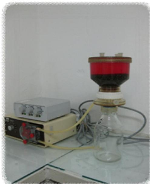
Fig.2. Biofilter with quartz sand for wastewater treatment in the textile industry [23]
