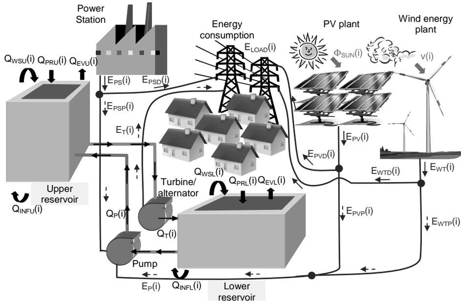
Fig. 10. Principle diagram of the renewable plant with characteristic elements
