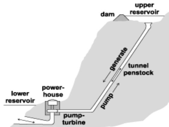
Fig. 3. Schematic of a conventional pumped-storage development with one reversible pump.
