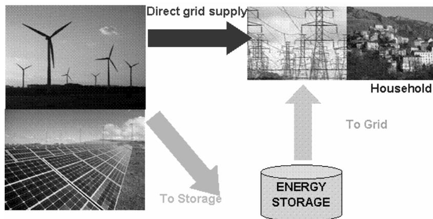
Fig. 8. Principle of coupling between renewable energy sources and hydro-pumped system.
