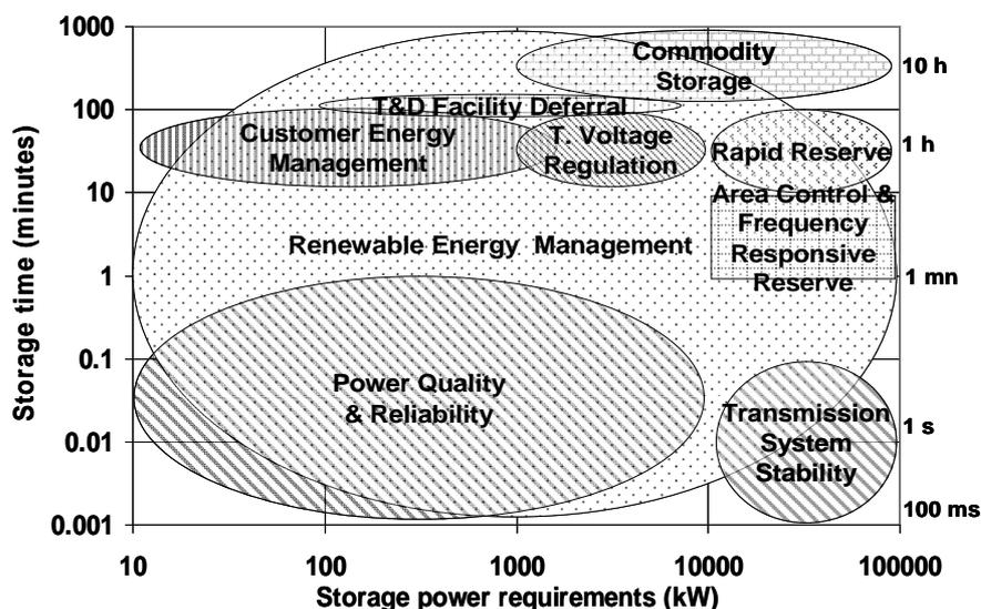
Fig. 1. Power and discharge time requirements for a variety of storage applications
